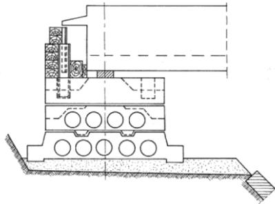
Fig. 16. Concrete element bank support (type KO-Pb) ('Central Office', 1997; Miklin & Sawicki, 1993)
