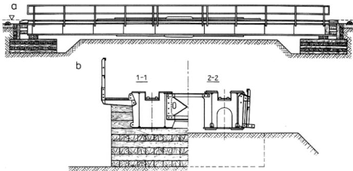
Fig. 14. Bridge-type stress-relieving structure; two box girder system type KO-21/73 ('Central Office', 1997; Miklin & Sawicki, 1993): a - longitudinal view, b - cross-section, 1-1 cross-section at support with folded pavement, 2-2 cross-section in the span with folded pavement
