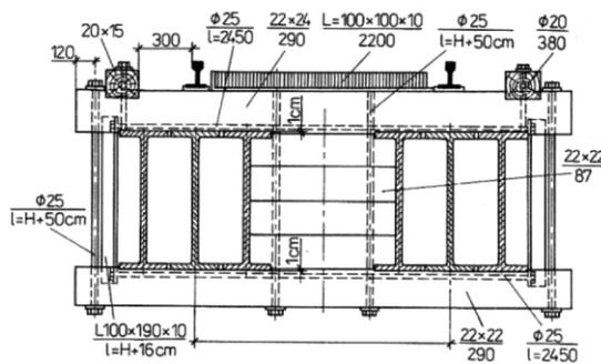
Fig. 10. Cross-section through a temporary span with steel girders constructed from three wide-flange I-beams (Cholewo & Szurowski, 1970; Miklin & Sawicki, 1993)
