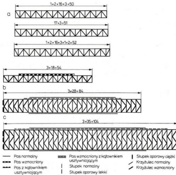
Fig. 4. Diagrams of the main girders in the spans of folding bridges of the R70 system (Białobrzeski, 1978; Miklin & Sawicki, 1993): a - single-storey girders, b - two-storey girders, c - three-storey girders.
