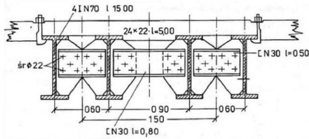
Fig. 9. Cross-section through a temporary span with steel girders constructed from two I-beams and with steel cross-bracing (Cholewo & Szurowski, 1970; Miklin & Sawicki, 1993)
