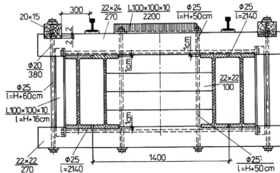
Fig. 8. Cross-section through a temporary span with steel girders constructed from two wide-flange I-beams (Cholewo & Szurowski, 1970; Miklin & Sawicki, 1993)
