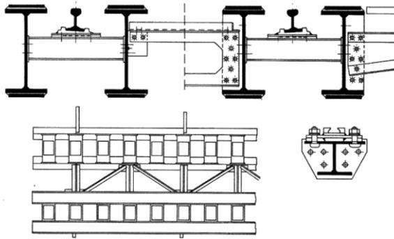
Fig. 13. Bridge-type relief structure; main girders composed of twin beams (Miklin & Sawicki, 1993; Rybak, 1982)
