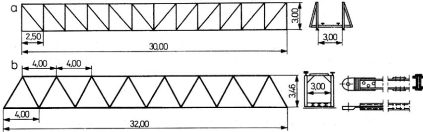
Fig. 2. Examples of lattice spans of collapsible bridges (Białobrzeski, 1978; Miklin & Sawicki, 1993): a - L30 system, b - L32 system
