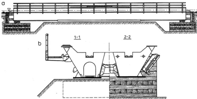
Fig. 15. Bridge-type stress-relieving structure; box span of the twin-beam system, type KO-30/75 (Miklin & Sawicki, 1993): a - longitudinal view, b - cross-section, 1-1 cross-section in the span with folded pavement, 2-2 cross-section at the support with folded pavement
