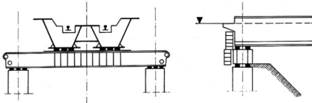
Fig. 18. Steel abutment founded on large diameter piles (type KO-Os) ('Central Office', 1997; Miklin & Sawicki, 1993): left - cross-section through the span at the support; right - longitudinal view of a section of the span
