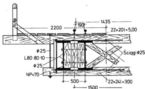
Fig. 6. Cross-section through a section of a temporary span with steel girders (each girder composed of two I-beams), with timber braces, bolted together (Cholewo & Sznurowski, 1970; Miklin & Sawicki, 1993)
