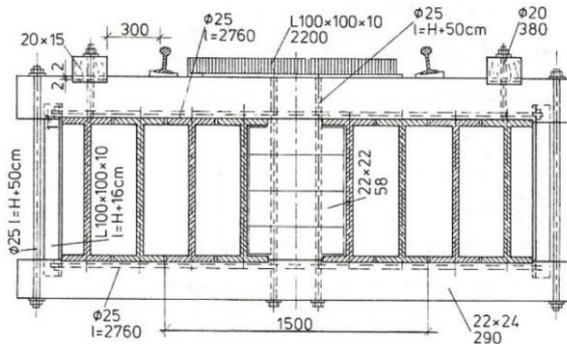
Fig. 11. Cross-section through a temporary span with steel girders constructed from four wide-flange I-beams (Cholewo & Szurowski, 1970; Miklin & Sawicki, 1993)
