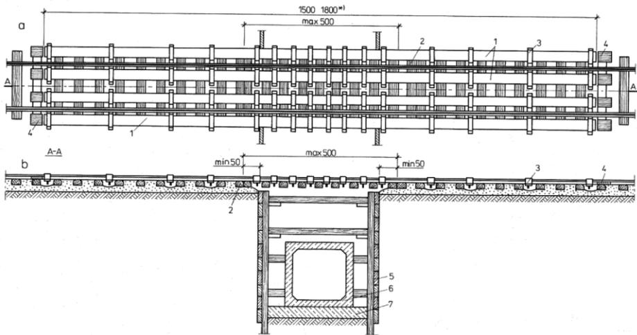
Fig. 21. Scheme of a rail relief structure for a concrete culvert reconstruction (Miklin & Sawicki, 1993): a - top view, b - cross-section through the reconstructed culvert, 1 - rail bundles, 2 - support sleepers in the obstruction zone, 3 - steel ties (chinstraps), 4 - timber blocks at the ends of the relieving structure, 5 - excavation formwork, 6 - reconstructed culvert structure, 7 - culvert foundation
