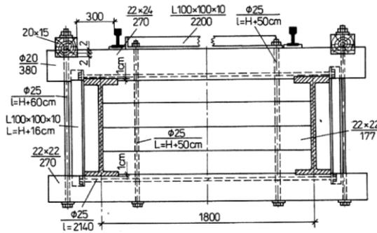
Fig. 7. Cross-section through a temporary span with steel girders constructed from single wide-flange I-beams (Cholewo & Szurowski, 1970; Miklin & Sawicki, 1993)
