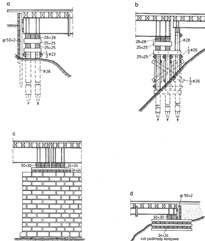
Fig. 19. Methods of supporting bridge-type relieving structures (Miklin & Sawicki, 1993): a - abutment made of a wooden yoke, b - intermediate support (pillar) for load-bearing structures with different span heights, c - support of the load-bearing structure on a fixed pillar, d - abutment as a cage made of railway sleepers
