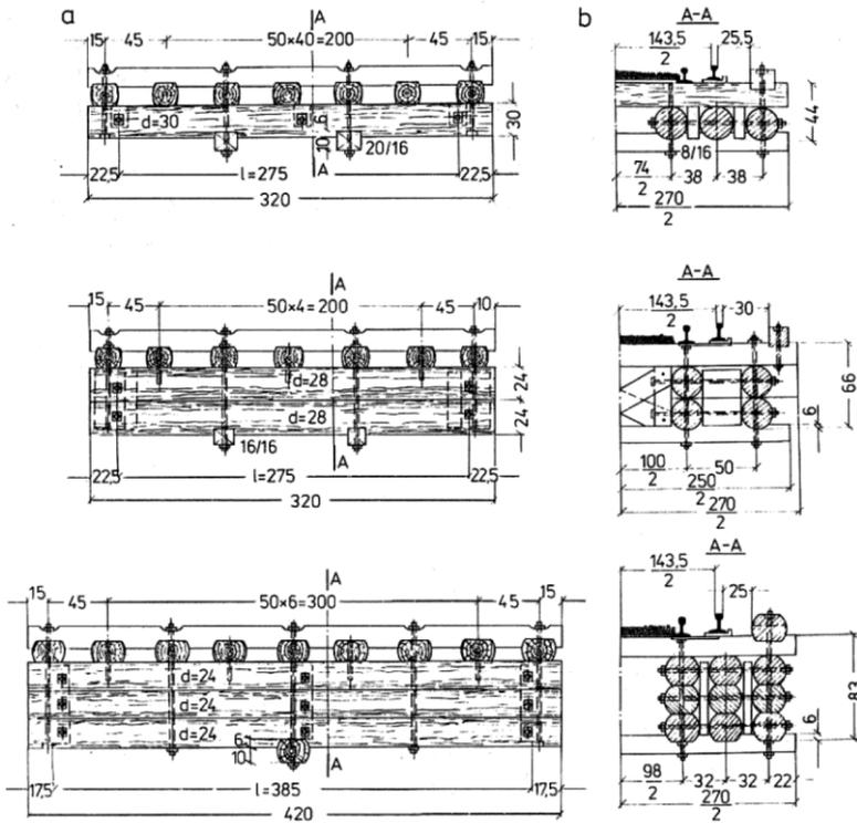
Fig. 24. Wooden spans of temporary bridges with main girders composed of so-called multiple beams (Cholewo & Szurowski, 1970; Miklin & Sawicki, 1993): a - longitudinal view, b - cross sections through a main girder composed of three, four and nine beams
