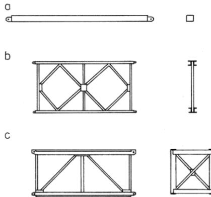
Fig. 1. Basic elements of a collapsible bridge (Białobrzewski, 1978; Miklin & Sawicki, 1993): a - linear element, b - planar element, c - spatial element
