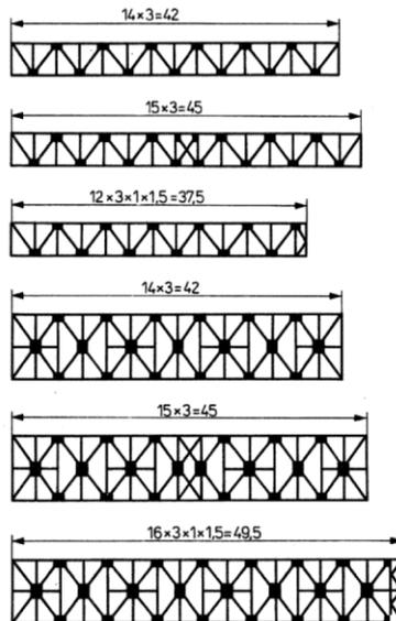
Fig. 3. Diagrams of the main girders in the spans of R-W system folding bridges (Białobrzeski, 1978; Miklin & Sawicki, 1993)
