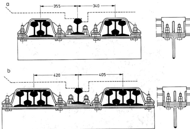
Fig. 22. Relieving structures composed of Swiss-type rail bundles suspended by stirrups (Miklin & Sawicki, 1993): a - three-rail bundle structure for obstacle span  $L_p \leq 3.0$  m; b - five-rail bundle structure for obstacle span  $L_p > 3.0$  m
