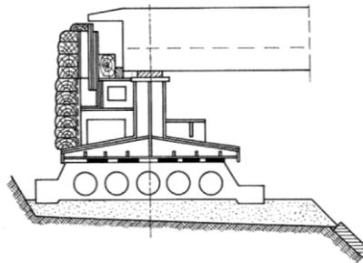
Fig. 17. Steel element bank support (type KO-Ps) ('Central Office', 1997; Miklin & Sawicki, 1993)
