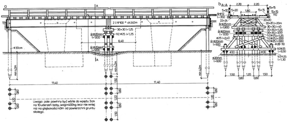
Fig. 12. Bridge-type stress-relieving structure of I-beams. Relieved track section 6.40 m long in the light of the abutments (indicated by the dashed line) (Cholewo & Sznurowski, 1970; Miklin & Sawicki, 1993); a - longitudinal view and location of foundation piles, b - cross-section A-A
