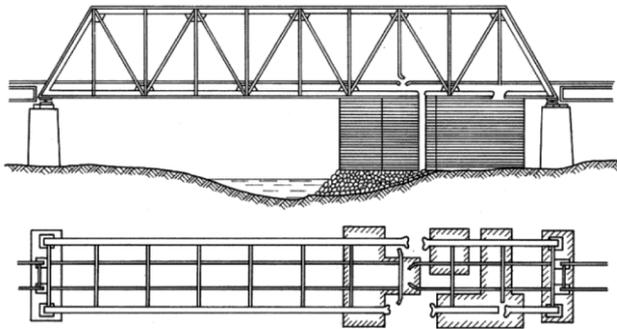
Fig. 10. Method of ad hoc reconstruction of a damaged truss with a bottom ride using additional supports constructed as cages from railway sleepers (Miklin & Sawicki, 1993)
