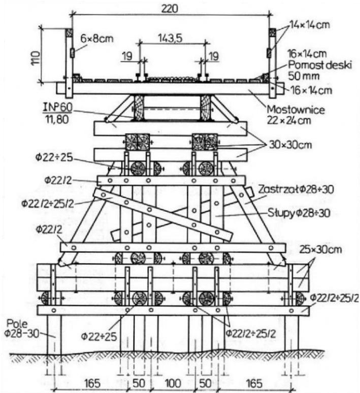
Fig. 6. Provisional bridge (Cholewo & Sznurowski, 1970): top – longitudinal view, bottom – AA cross-section through the bridge pillar
