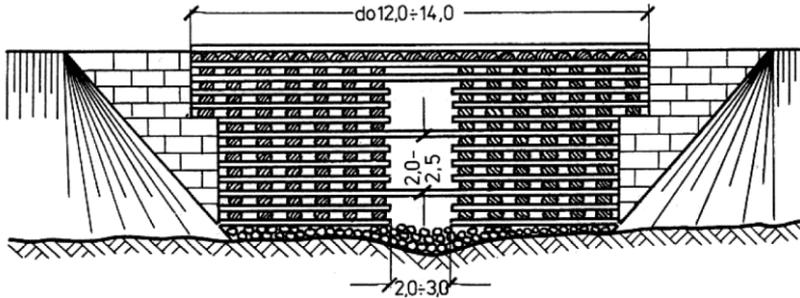
Fig. 2. Filling the opening of a damaged bridge using a structure in the form of ‘cages’ made of railway sleepers (Cholewo & Szurowski, 1970; Miklin & Sawicki, 1993)
