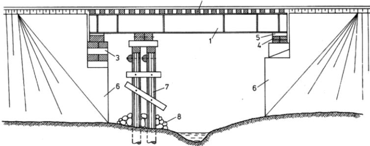
Fig. 9. Reconstruction of a single-span bridge (Miklin & Sawicki, 1993): 1 – bridge span raised to its original position, 2 – railway superstructure, 3 – hardwood packs, 4 – steel ties, 5 – steel washers, 6 – bridge abutment bodies, 7 – additional pile support due to weakening of the span structure, 8 – armour rock.
