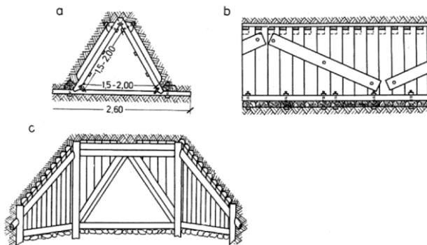
Fig. 1. Provisional culvert with a triangular cross-section made of railway sleepers (Cholewo & Szurowski, 1970; Miklin & Sawicki, 1993): a – cross-section, b – side wall reinforcement, c – view from the inlet to the culvert
