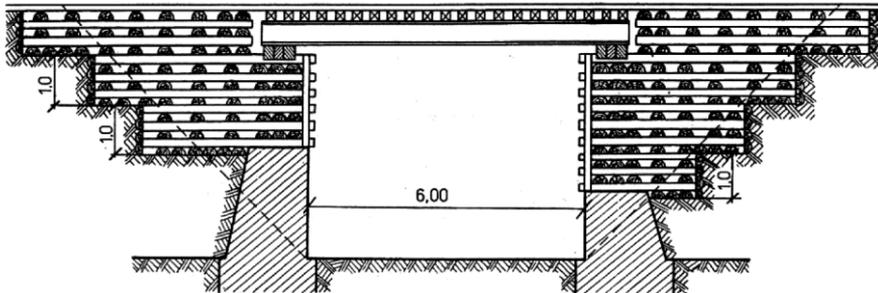
Fig. 4. Provisional reconstruction of a bridge with a span made of I-beams on supports (abutments) made of railway sleepers forming so-called cages (Cholewo & Szurowski, 1970; Miklin & Sawicki, 1993)
