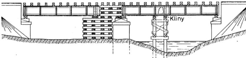
Fig. 8. Provisional reconstruction of a two-span bridge using damaged plate girders (right span) (Cholewo & Szurowski, 1970; Miklin & Sawicki, 1993)
