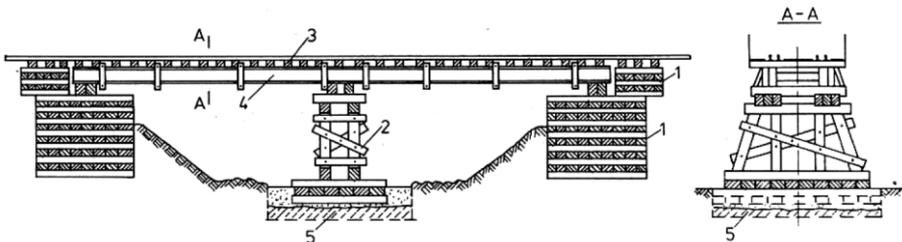
Fig. 3. Provisional bridge reconstruction (Cholewo & Szurowski, 1970; Miklin & Sawicki, 1993): 1 – railway sleeper cages forming the bridge abutments, 2 – provisional support in the form of a wooden yoke, 3 – railway pavement, 4 – provisional span, 5 – substructure of the intermediate support in place of the destroyed pillar of the fixed bridge
