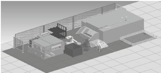
Fig. 8. Concept of an automated final assembly cell.
