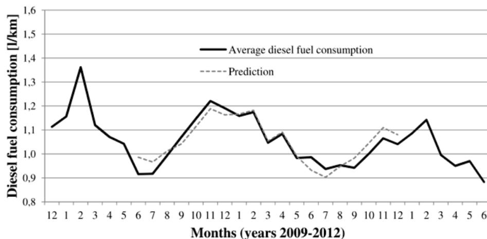
Fig. 5. The graph matching of prognostic model of diesel fuel consumption by railbuses based on seasonal indicators.
